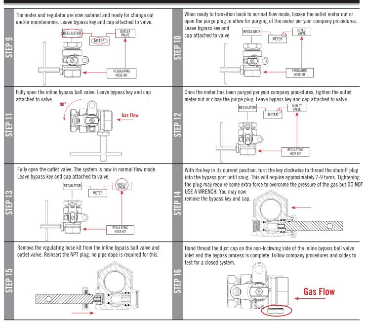
Inline bypass valves are operated by a proprietary pentagon key supplied by A.Y. McDonald.
